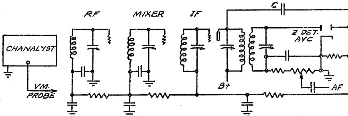
The voltmeter probe is connected to the AVC bus or to the grid of one of the controlled tubes.
