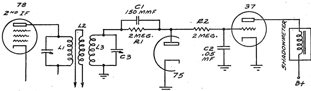
FIG. 8.—Shadowmeter circuit of the Philco model 201.
