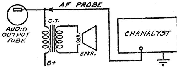
The AF Channel probe is connected to the output tube plate or to some other point in the audio system.
