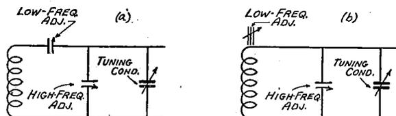
In (a) the low frequency adjustment is accomplished by means of a trimmer condenser while in (b) a movable iron core is used.
