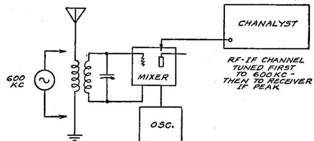
The RF-IF probe is used when aligning the r-f system and also when adjusting the oscillator padder.
