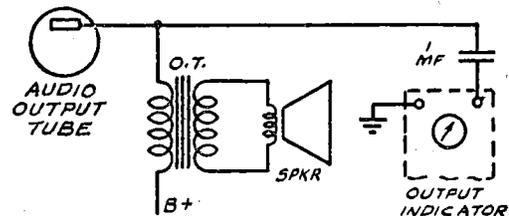
By determining the maximum audio output of a super-heterodyne with an a-c voltmeter, the correct adjustments of the various trimmers are found.
