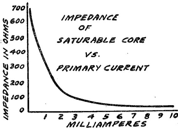
Fig. 15.—Variation of core saturation with primary current.
